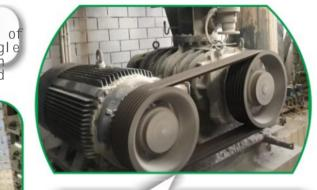
The original vacuum system of this company runs 5 Roots vacuum PumPs, supporting the motor Power of 560kW the actual operating Power of 430.53kW, the original equipment due to long running time. old equipment. resulting in high energy consumption a large waste of lectricity resources. In order to further improve the operating efficiency of the company, the company upgraded the five Roots vacuum pumps.
