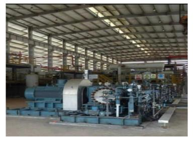
The first commercial hydrogen energy project in China 32MPa hydrogen filling compressor
